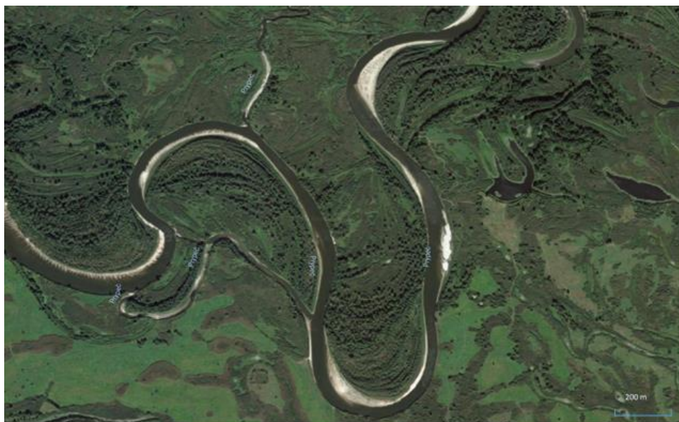
Fig. 2.2 Meanders of Pripyat in the Pripyat National Park. Radius of meanders is smaller than 200 m, which can pose significant risk in navigation of the ships longer than 50 m. Orthophoto: Google.
